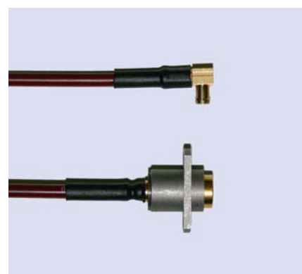
Kabel / Cable Anschluß Connector Succoform 86 FEP/PE MCX-Winkelstecker/BMA-Einbaukuppler MCX angle male/BMA bulkhead female
