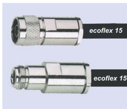
Kabel / Cable Anschluß Connector ECOFLEX 15 N-Stecker/N-Kuppler N male/N female
