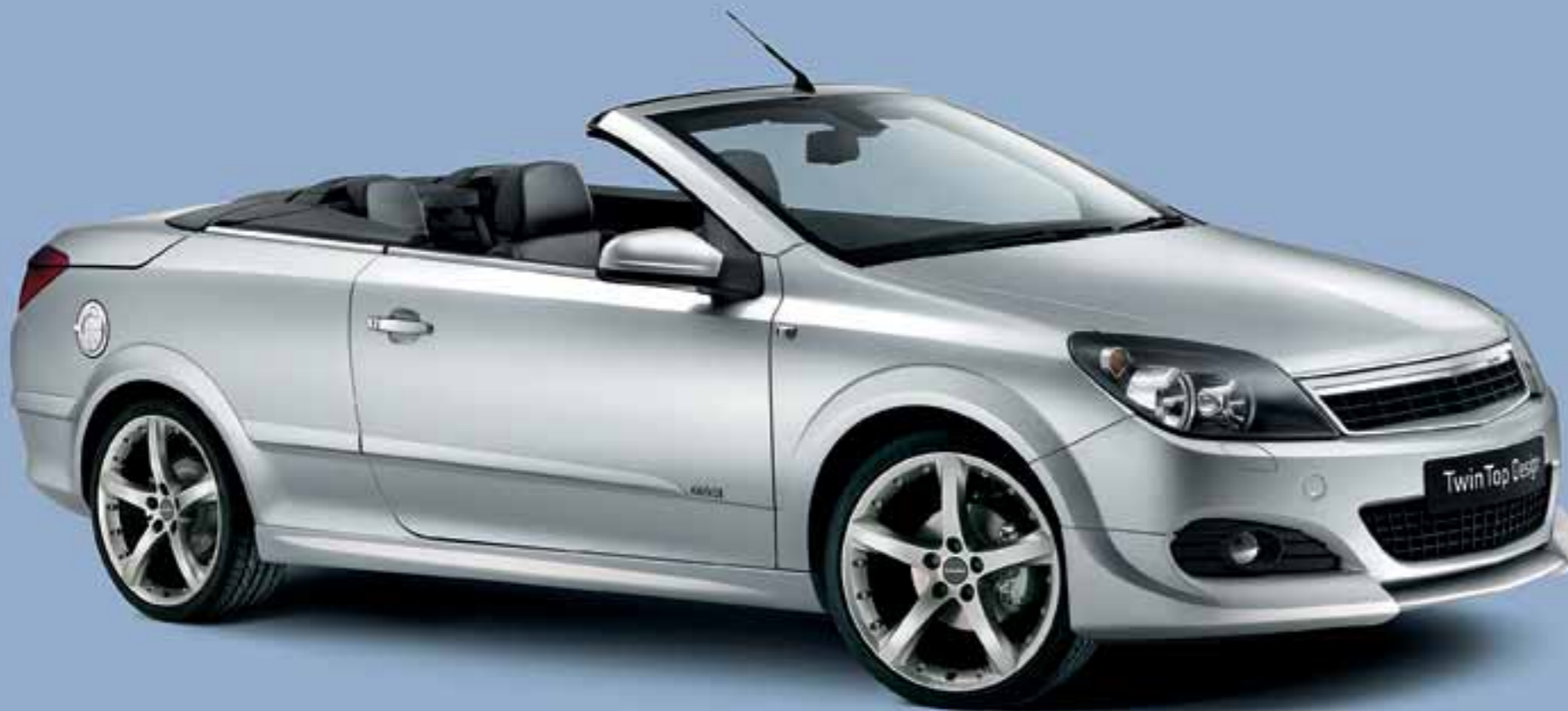
Design model illustrated features Irmischer front lower skirt extensions, cross hatch grille with aluminium upper and laser-etched 'Irmischer' badge, side sills, stainless steel door handle covers, aluminium-effect fuel flap cover and 19-inch GT star 'titanium effect' alloy wheels.
